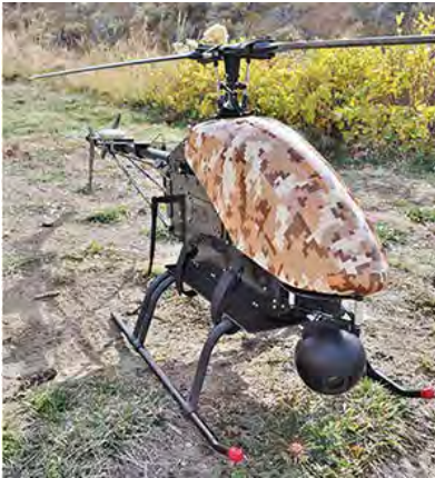
Figure 3: Leptron Avenger UAS Helicopter with manufacturer specifications. http://www.leptron.com/leptron_avenqer_uas_helicopter.html
